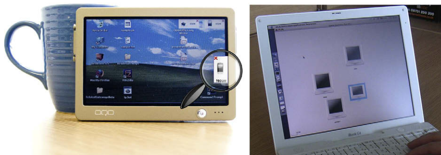
Fig. 6 – Integration of spatial references to near-by devices in the mobile user interface; left, extension of Guinard et al.'s (2007) Gateways ; right, Kortuem et al.'s (2005) map view.
