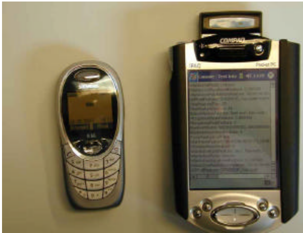
Fig. 2 Feature extraction on a typical PDA with a mobile phone as additional sensor
